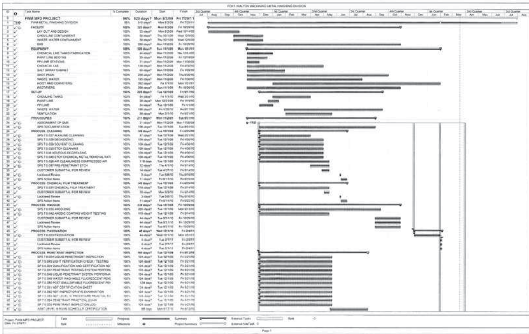
FIGURE 4.8 Combined WBS & Gantt chart schedule format. Courtesy of Fort Walton Machining, Inc.
